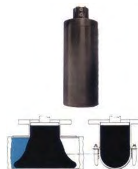
Expandable stoppers for water use in cast and ductile iron, PVC and steel pipe. Size range: 8" – 20" (200mm – 500mm). Rate to 250 PSI (17bar). Larger sizes available.
